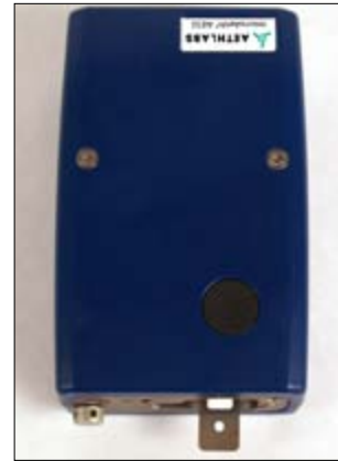
Figure 6: Bottom of AE51 with filter strip release button.
