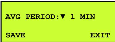
Although the E-Sampler measures the particulate concentration and updates the display each second, the fastest average period that can be logged in memory is 1 minute. The 1 second concentration can be output and logged externally using the E-Sampler analog output.
