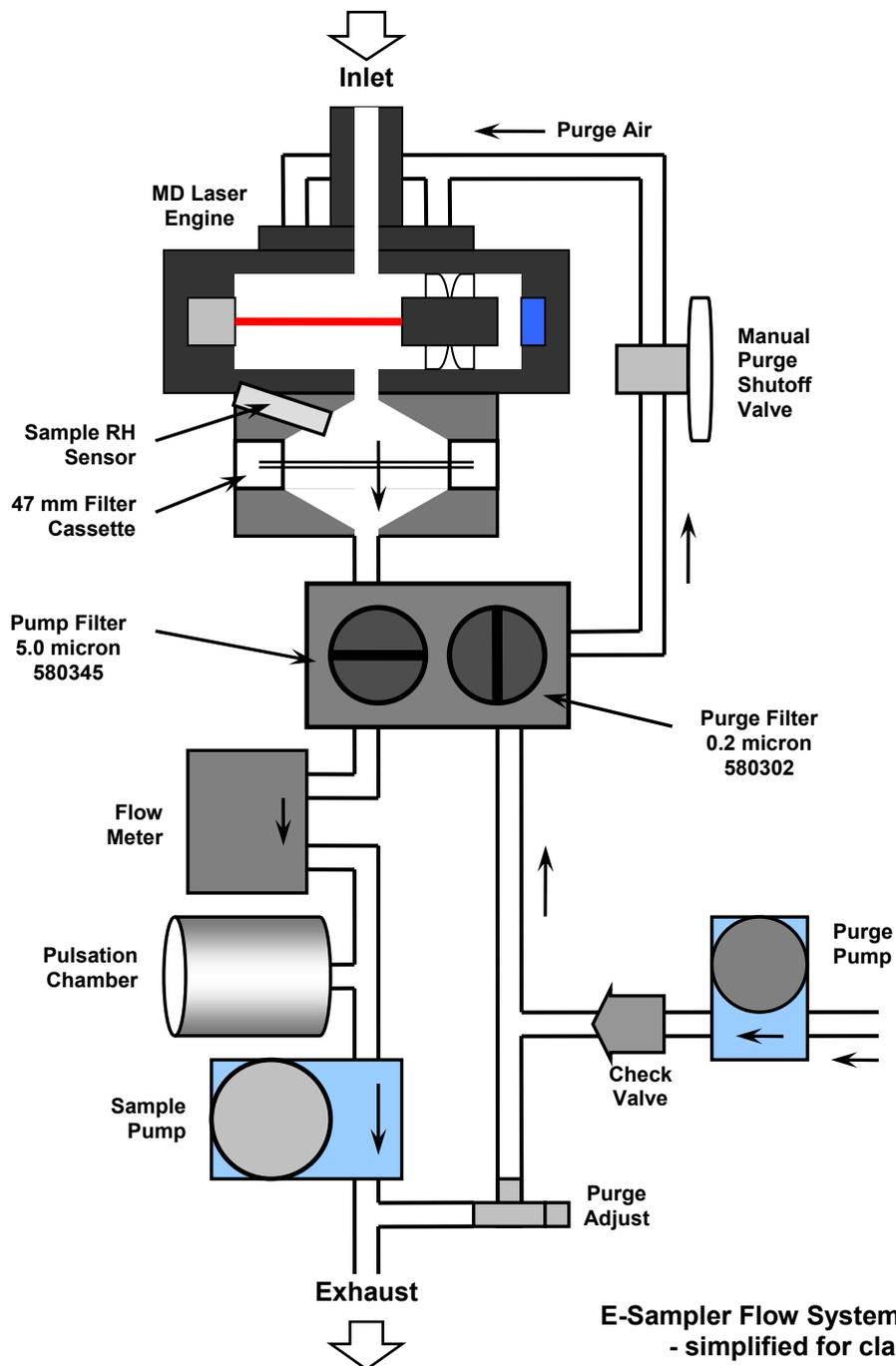
**E-Sampler Flow System Diagram
