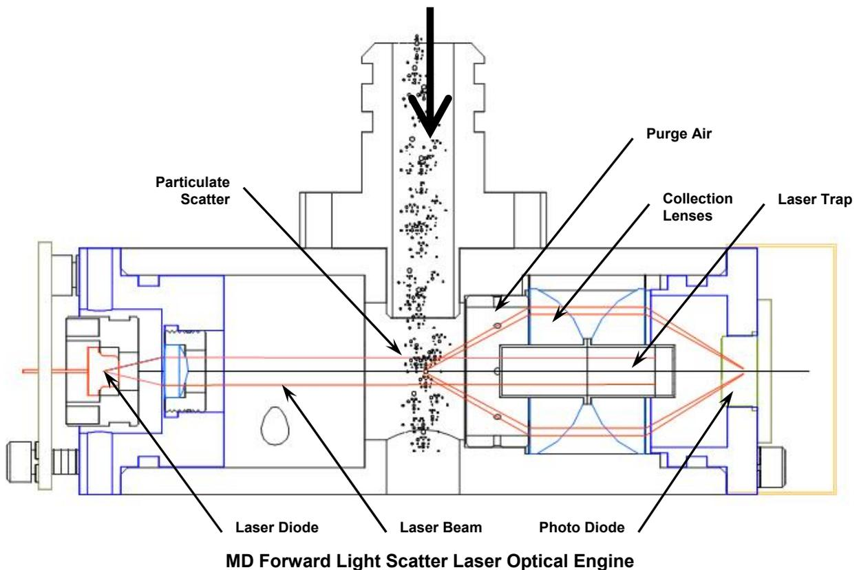
Forty detector measurements are made and averaged into an updated concentration value each second. These 1-second values are temperature compensated using a factory-set algorithm, and averaged into the user-selected data storage interval of 1, 5, 10, 15, or 30 minutes. The 1-second values are also displayed on the LCD and available on the analog output.
