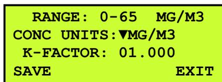
The RANGE value is the full-scale range of the E-Sampler analog output. Units with firmware R2.0.0 and later have a fixed range value of 65mg, with a separate analog range setting in the communications setup screen, Section 6.8.
