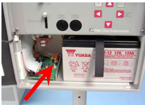
**Internal battery and 81220 PCB battery harness connection**
