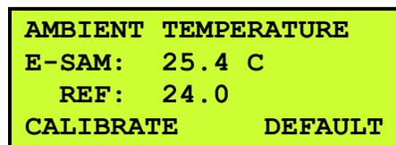
The E-SAM parameter is the current reading from the E-Sampler temperature sensor. The REF parameter is where you can enter the correct value from your traceable temperature standard, using the arrow keys. The E-SAM value should change to match the REF value when you press the CALIBRATE soft key.
