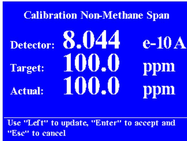
**Figure 8 Calibration. non methane span screen**
