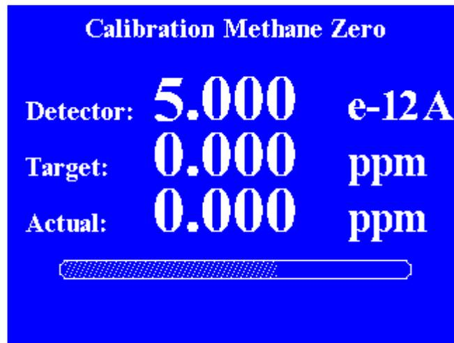
**Figure 9 Auto calibration methane zero screen**
