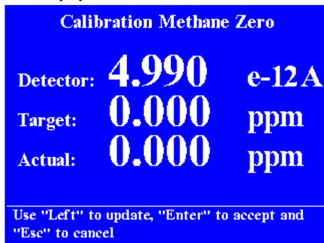
Figure 5 Calibration. methane zero screen
