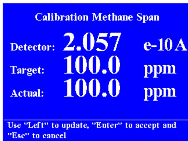
**Figure 6 Calibration methane span screen**
