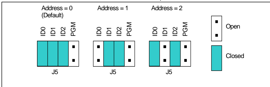
Figure 4. 9400TPIM (J5), Hardware Address Jumper Configuration.
