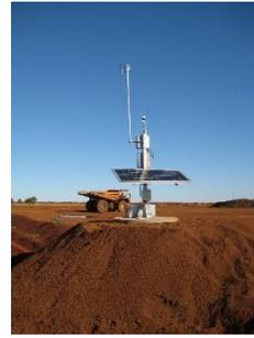
*Solar powered particulate monitor on a mine site in Western Australia.*
